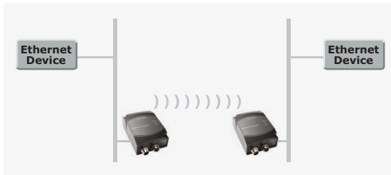
Ethernet Port Adapters (EPA) replacing the ethernet cable with wireless connection.
