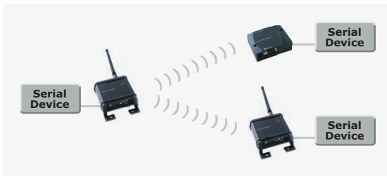
Serial Port Adapters (SPA) replacing the serial cables with wireless connections in point-to-point and multidrop setups.
